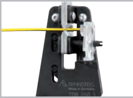
Precise cutting of the insulation to a complete extent.
