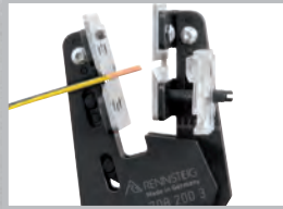
Automatic stripping of the insulation.
