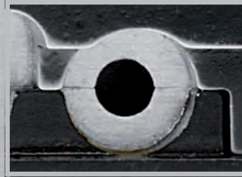
Stripping Area (Round Blades, no wire damage)
